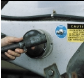
Independent earthing connection
