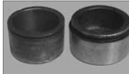
Early type front piston to the left, diameter 48 mm. Metric type 16 piston to the right, diameter 54 mm. Observe the different grooves for the rubber gaiter. The later type piston to the right, has a newer and more effective type of groove, that will neither fit with the original gaiter nor original caliper.
