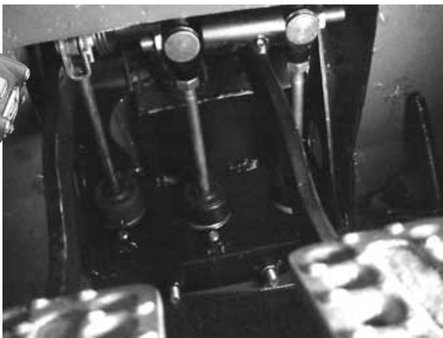
Brake balance bar photographed in place. At the left in the photo the clutch master cylinder can be seen, then the pair of brake master cylinders and the balance bar adjusted with the longest stroke to the master cylinder of the rear circuit.
