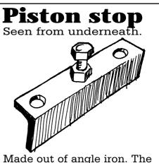
Made out of angle iron. The bolt is held in place by two nuts and constitutes the actual stop for the piston.
