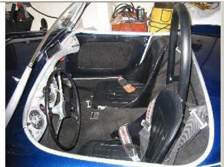
Cockpit with new centered hoop roll bar
