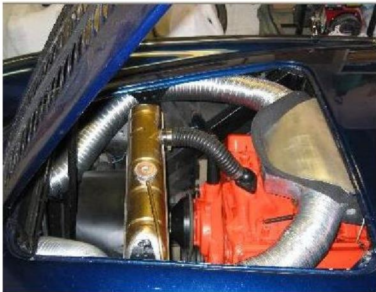
Engine compartment with 4in OAI ducting
