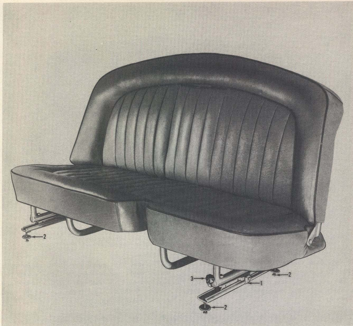
FIGURE 27-C—Front Seat Assembly and Adjuster Tracks.
