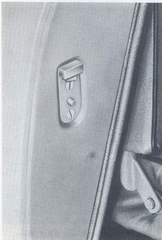
FIGURE 22—Door Lock Striker and Dovetail Assembly Right Side Shown.
