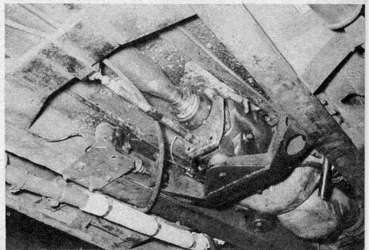
Above: Rear transmission mount, fabricated from 3/10-inch steel, employs both Ford and Chrysler front mounts. Sloppy shift action eventually caused owner to switch to '37 Buick top-shift box (right) eliminating need for extra linkage. The steady rod, set between box and cross-member, was beefed-up.
