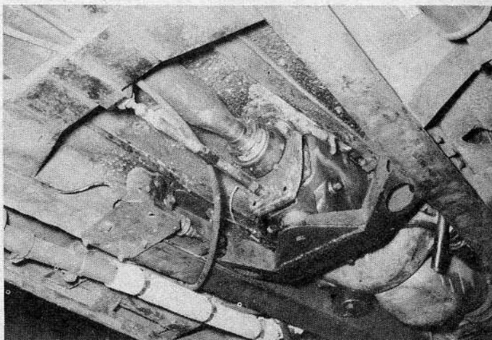
Above: Rear transmission mount, fabricated from 3/10-inch steel, employs both Ford and Chrysler front mounts. Sloppy shift action eventually caused owner to switch to '37 Buick top-shift box (right) eliminating need for extra linkage. The steady rod, set between box and cross-member, was beefed-up.
