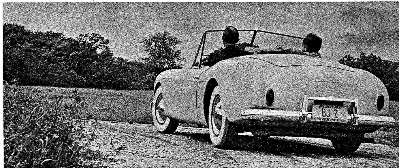
Streetable 1951 N-H used coil springs all around, trailing links up front, carried 16-gal. tank. Wheelbase was 102 in., and overdrive was standard.
