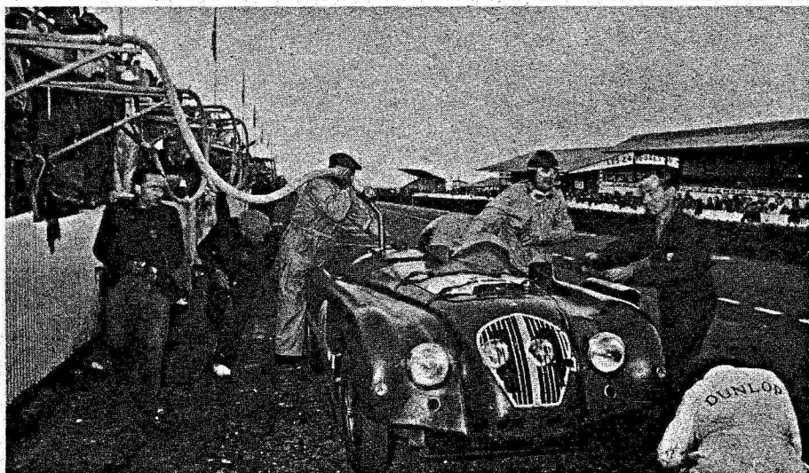
Gassing up—this car was driven by Veyron and Giraud-Cabantous in 1953, fitted with the Sampietro head. Output stood around 200 bhp, but car konked out early; another N-H placed 11th.
